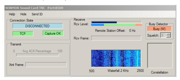
The "Busy Detector" on the TNC display should tell you if the channel is busy or clear, but it is often confused by noise, so it's best to look at the waterfall display to see if a signal is visible. If the channel is busy, either wait for the other station to finish or select a different channel.
