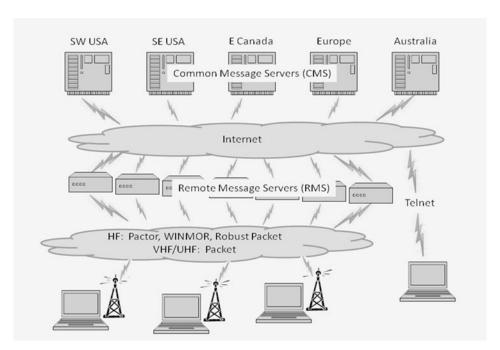
The Winlink system consists of a group of Common Message Servers (CMS) placed at various locations around the world. These servers connect via the Internet to Radio Message Servers (RMS) in many geographic locations to form a star network configuration. The Radio Message Servers are the VHF, UHF, or HF RF gateway into the Winlink system. The final component is the client computer (i.e., your computer) which runs software to send/receive messages through your radio.
