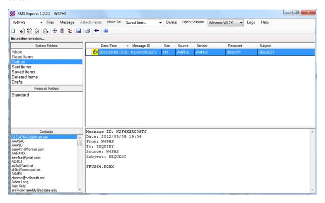
Next, open a session and connect to an RMS server to send the query request. After a few minutes, the Winlink system will process your request and post a reply message that you can receive by connecting to an RMS server and receiving incoming messages.
