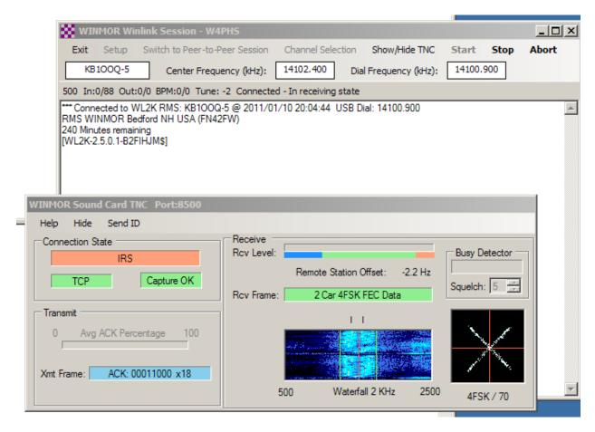
If you can't connect, try a different channel. If you do connect, watch the "Rcv Level" bar at the top of the TNC screen to make sure your received audio signal level is in the green zone. If it isn't, adjust the "RX" knob on the SignaLink to get it in the green region.
