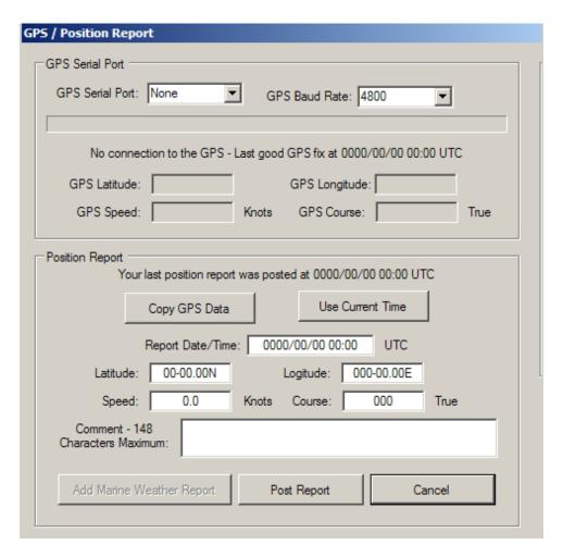
Select the COM port that your GPS unit is connected to in the "GPS serial port" list, and select the baud rate. The standard baud rate is 4800 baud.
