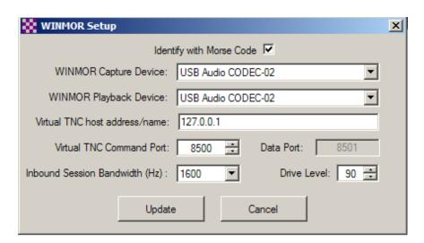
Select the sound card entry corresponding to the SignaLink in the WINMOR Capture and Playback fields; it will be labeled "USB Audio CODEC", but the number at the end may be different. For ham operation, check the box "Identify with Morse Code". Leave this box unchecked for MARS operation. After you finish filling in the soundcard information, click the "Update" button to save the information and close the screen.
