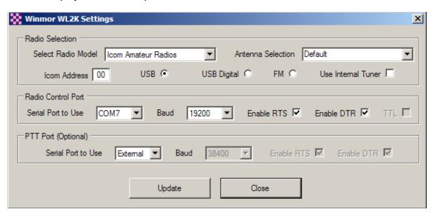
Open the "Select Radio Model" list and select the entry that is closest to the type of radio you have. Set the Radio Control Port fields to match the COM port and baud rate of your radio control interface. Set the PTT Port option to "External". If you don't have the ability to automatically control your radio, you can still use RMS Express. Just manually tune to the "dial frequency," and set USB SSB mode. Click Update to close the setup screen.
